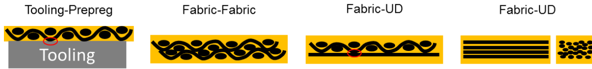
Figure 5. Influence of fiber architecture on the interaction with neighboring plies
