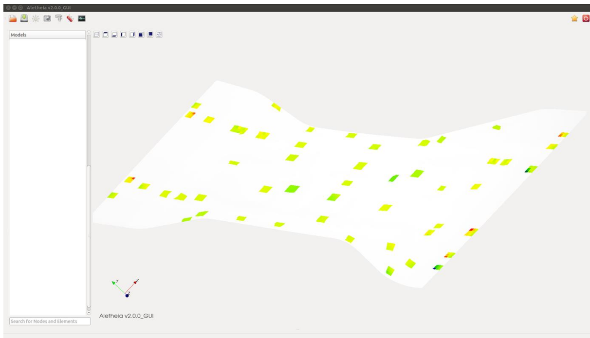
Figure 5. Visualization of the ratio between measured and predicted strains at the locations of the strain gauges of one selected component
