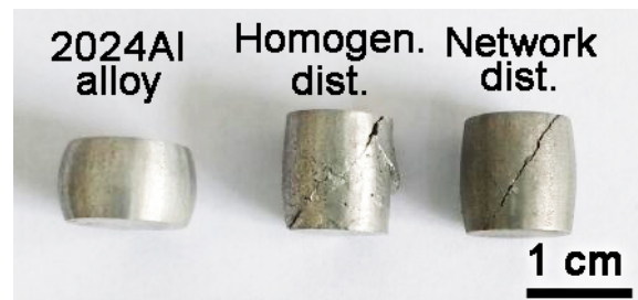
Figure 6 Photographs of samples after compression test (a) Unreinforced 2024Al alloy (b) 10 vol.% homogeneous composite and (c) 10 vol.% network structured composite.
