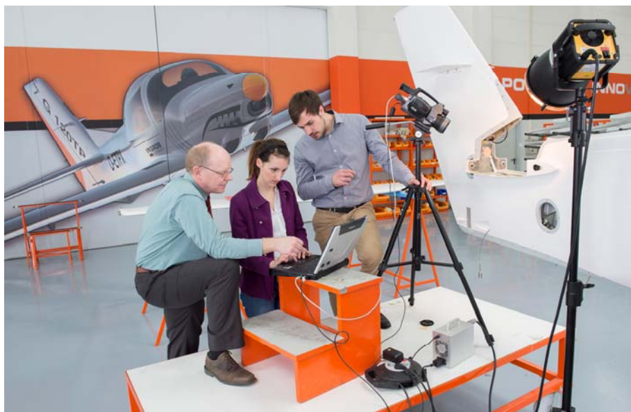
Figure 3. Optical lockin thermography at an empennage (© Werner Bachmeier, TU München)
