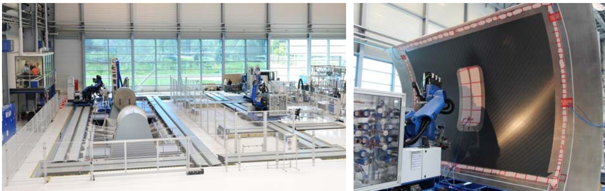
Figure 1. Left: Overview of the GroFi plant. Right: production of a fuselage skin with AFP technology.
