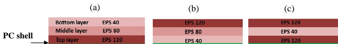
**Figure 1.** Three different configurations of composite foams (a), B40/80/120T; (b), B120/80/40T; (c), B120/40/120T.
