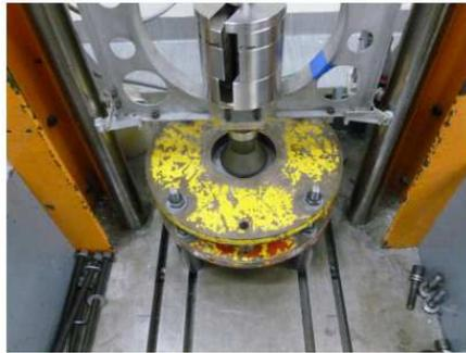
Figure 3. Linear drop weight impact set-up with flat steel tub on a foam+shell sample.
