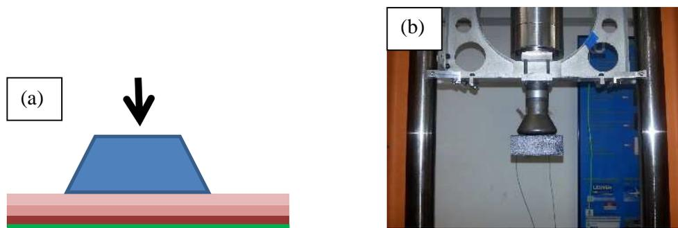
**Figure 2.** a) an illustration of a layered composite foam connected to impact tub; b) an image of impact set up whilst the foam specimen connected to flat tub.
