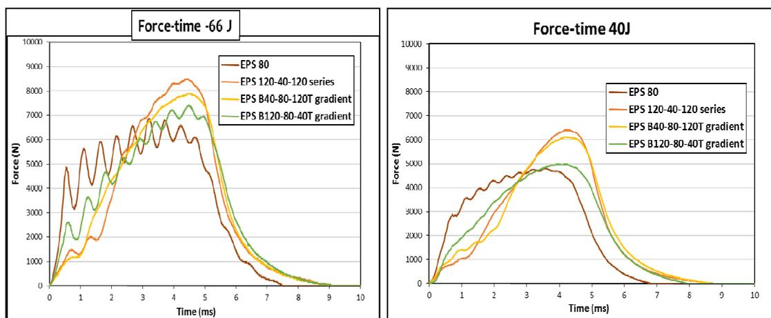
Figure 4. Force-time graph of different composite foams obtained from linear impact with initial energy of 66 J and 40 J.
