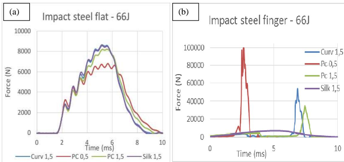
**Figure 5.** Linear impact force-time graphs with a) flat steel tub and, b) finger steel tub.
