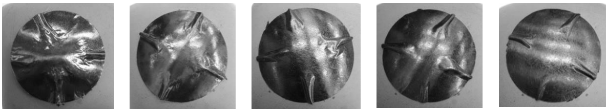
Figure 8. Results when forming [0.90, 45.135] preforms at different speeds, from left to right: fast (<0.5s), medium (10s), slow (1hr), very slow (2hr), and ultra-slow (20hr).
