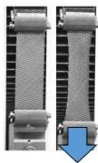
Figure 4. (Left) Bias extension test (showing different material to that used). (Right) Results showing the increased stiffness at higher deformation rates.
