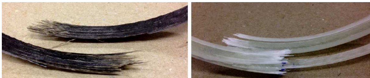
Figure 1. Fracture regions of ring segment specimens: basalt fiber composite B1 (left) and glass fiber composite G1 (right) reinforced composite.
