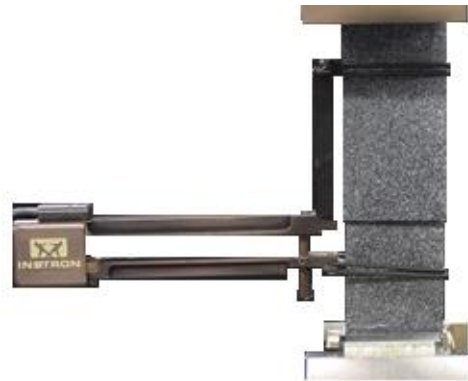
Figure 5 Single lap shear test setup
