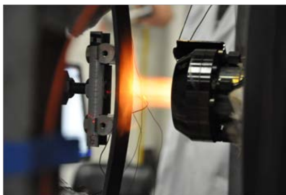
Photo 1 : Experimental device – Mechanical test of carbon epoxy laminate exposed to a methane burner flame
