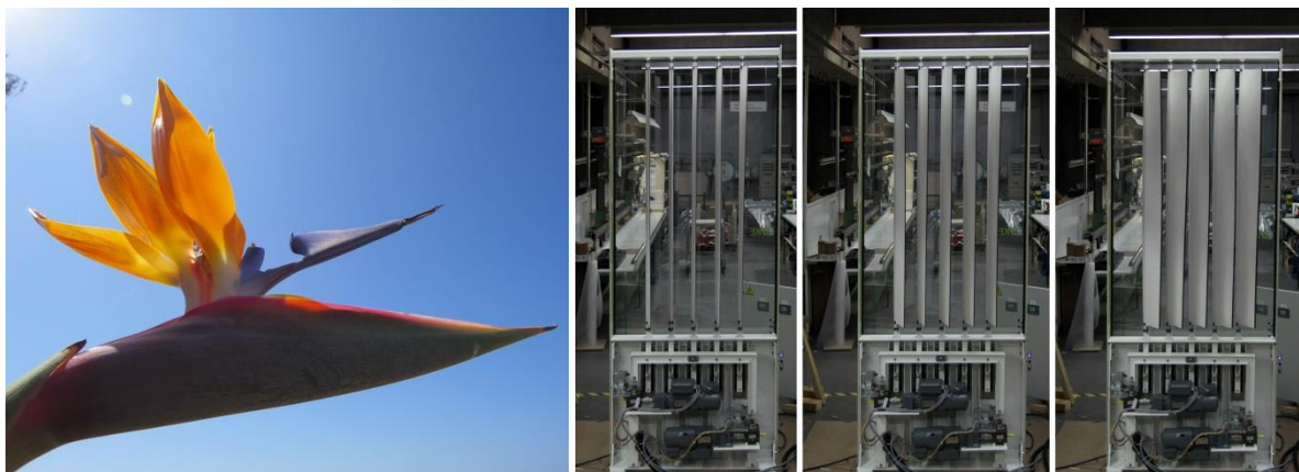
Figure 5. Flower stand of the bird-of-paradise flower with a violet perch acting as role model for the hingeless biomimetic façade-shading system flectofin®. Demonstrator of the biomimetic façade-shading system flectofin® actuated by bending of the backbone with hydraulic pistons at the base of each module in various states of closing, © Plant Biomechanics Group Freiburg, ITV Denkendorf & ITKE University of Stuttgart.
