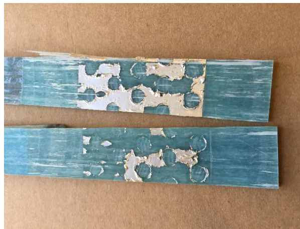
Figure 8. Significant tearing within patterned aluminium foil
