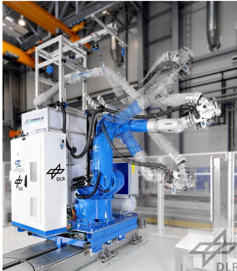
Figure 3. WingCover Dry Fiber Placement (DFP) Unit at DLR Stade
