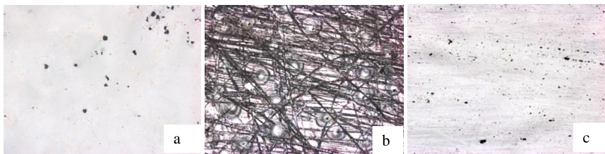
Figure 7. PU coating on metal sheet: virgin surface, b) scratched surface, b) scratched surface after healing treatment.
