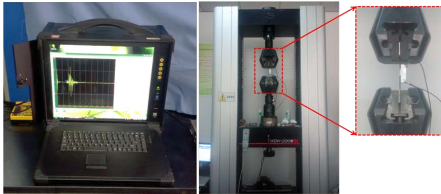
Figure 2. The measurement system of acoustoelastic coefficient.
