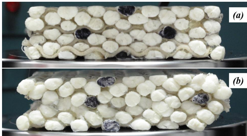
Figure 3. The final states of composites after compression: (a) Composite A; (b) Composite B.
