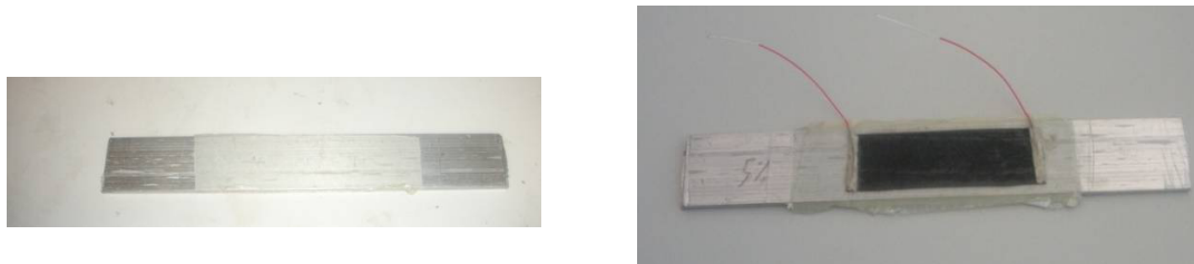
Fig. 9 Sample bonded on a rigid support
