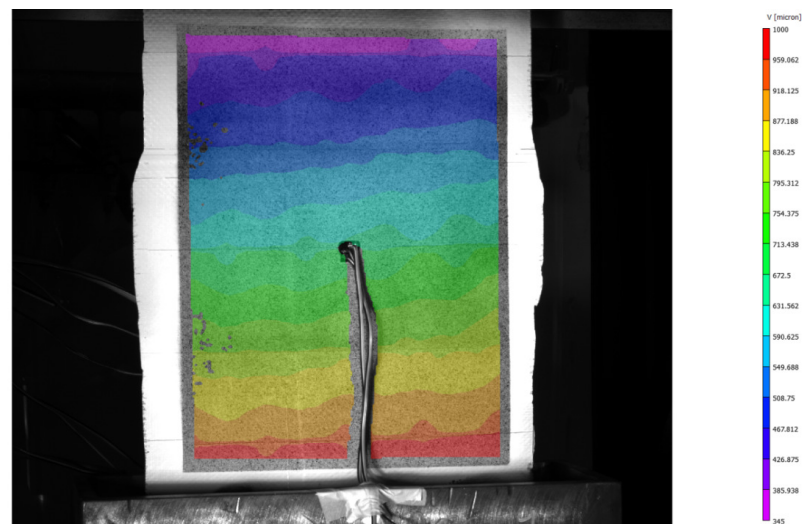
Figure 12. Axial displacement of the panel interpolated by means of DIC.
