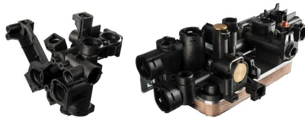
Figure 1. A complex injection molded thermoplastic flow block (left) and a hydroblock, assembled with a heat exchanger (right), made of NORYL™ resin (short glass fiber reinforced PPO™/PS).
