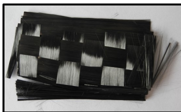
Figure 1. Recycled carbon fibers after the fiber-matrix separation process.
