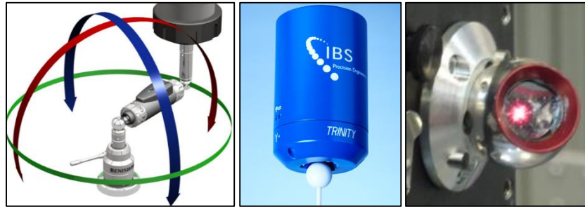
Figure 4. Left to Right; Renishaw Ballbar [6]. IBS Trinity Probe [7]. Lieca Laser Tracker SMR
