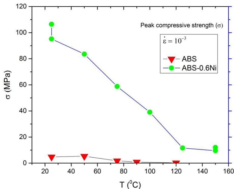
Figure 3. Strength of polymer (ABS) and the composite of 0.6 volume fraction of Nickel at different temperatures
