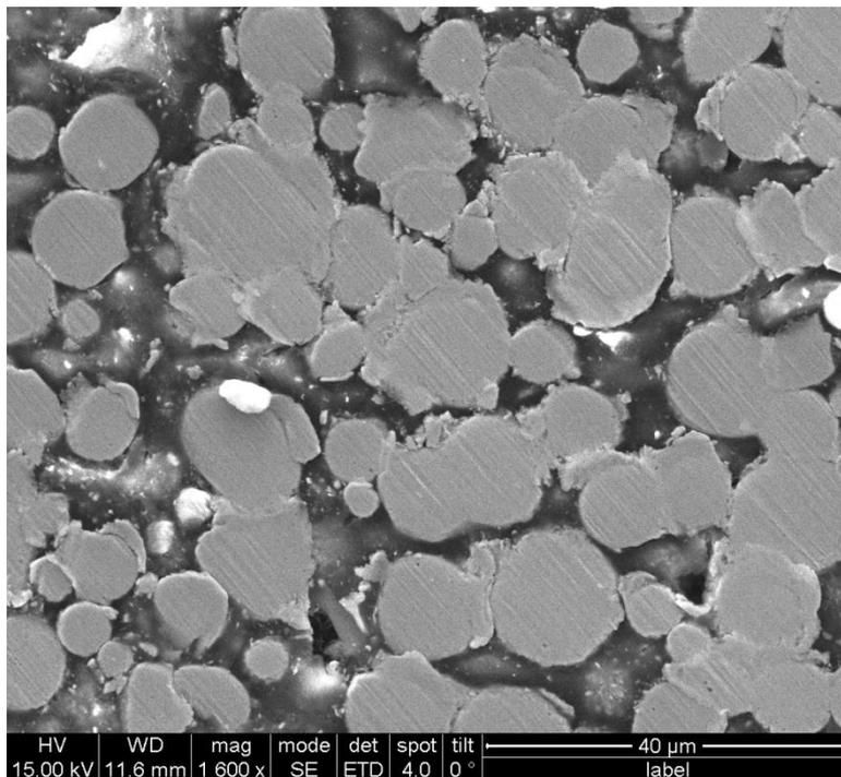
Figure 2. Scanning electron micrograph of the composite of 0.6 volume fraction of Nickel
