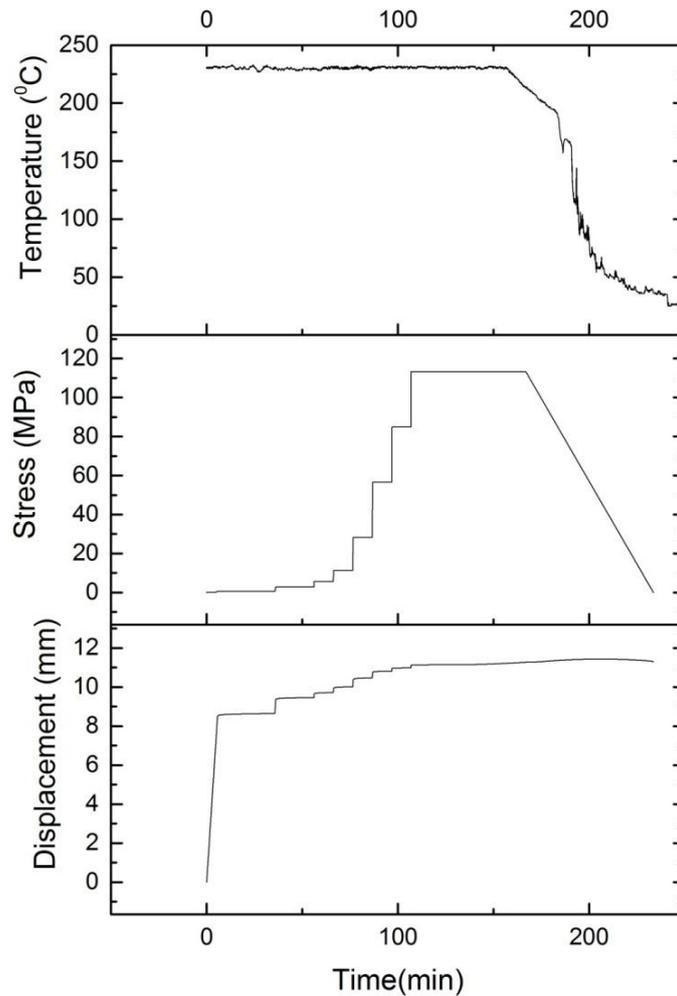
Figure 1. Processing parameters used for compaction
