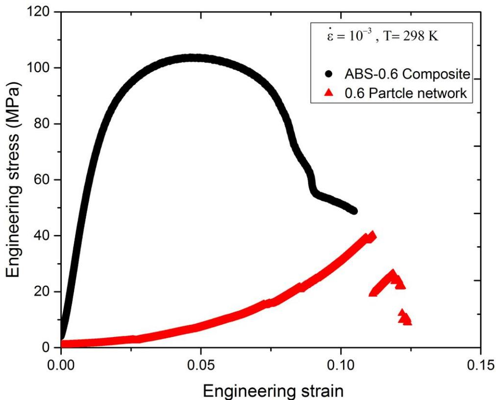
Figure 4. Comparison of compressive strength between the composite (0.6 volume fraction of nickel) and the left over particle network after burning off the polymer
