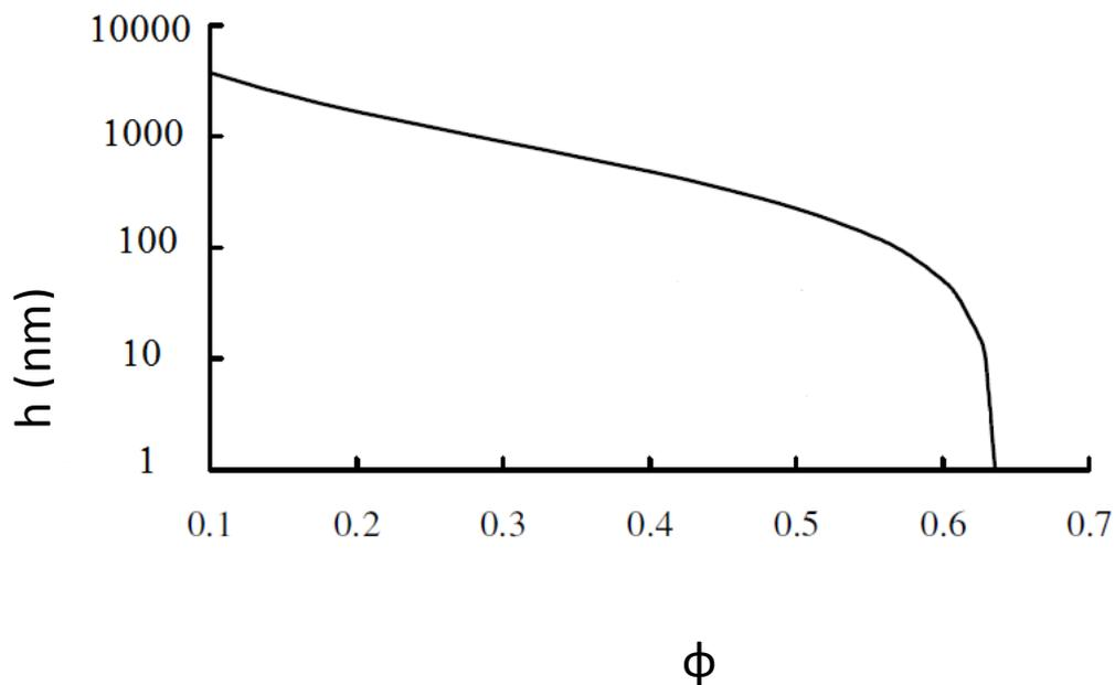
Figure 5. Average inter particle spacing (h) between two nearest particles of 10  $\mu\text{m}$  diameter with volume fraction( $\phi$ ) of particles (reproduced from [7])
