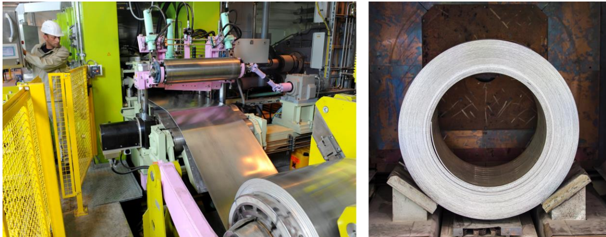
Figure 2. Four High Reversing mill at the TU Bergakademie Freiberg.
