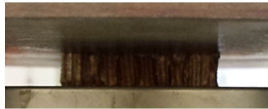
(d) Nomex core at failure point under compressive loading
