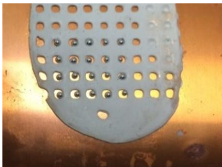
Figure 4. Macroporous polymer cages on a Mylar® dielectric coated copper plate filled with Hg droplets.
