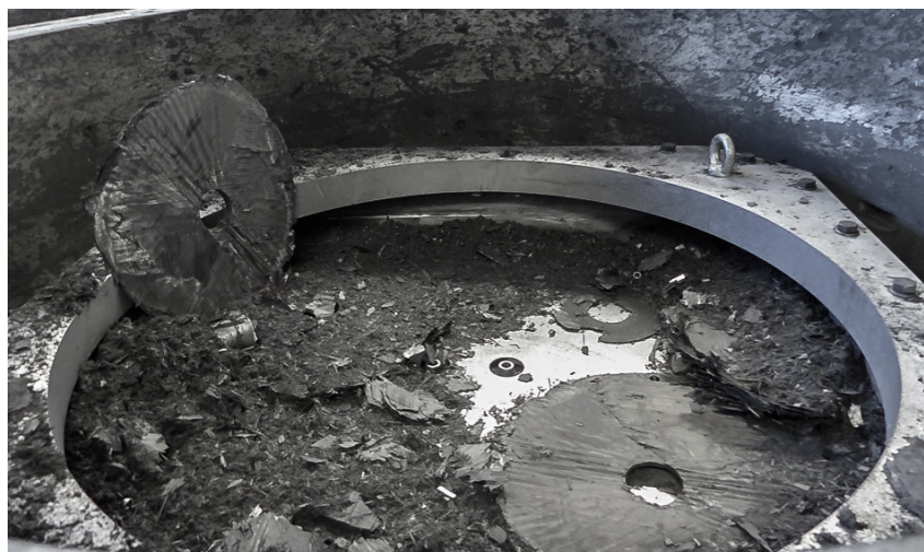
Figure 8. Destroyed chopper disk after spinning strength test.
