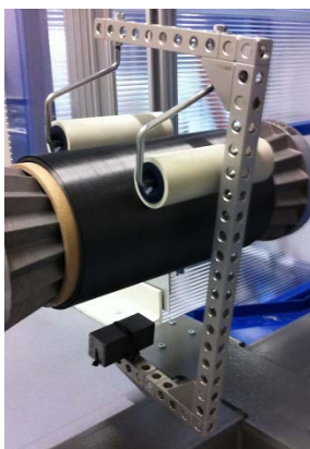
Figure 7: Example of a clamping mechanism to hold down bending resistant rolled goods like UD tape while being fed to the cutter.
