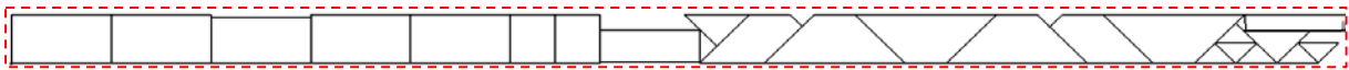
Figure 3: Nesting for a skin part preform out of sliced UD layers, material utilization degree \approx 95\% .
