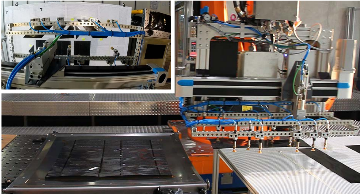
Figure 10: Robotic pick and place end-effector in robot cell (top left: on board view).
