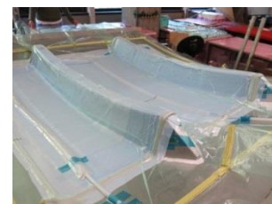
Figure 5. VAP infusion setup for 2 \Omega -frames
