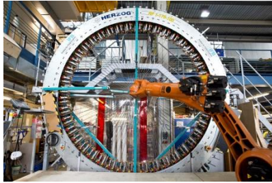
Figure 2. Radial braiding machine at IFB
