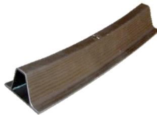
Figure 7. Impregnated \Omega -frame with bonded multiaxial fabric skin
