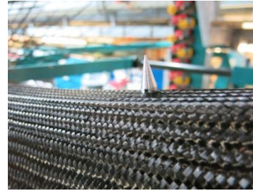
Figure 3. Overbraided mandrel with tapered displacement element
