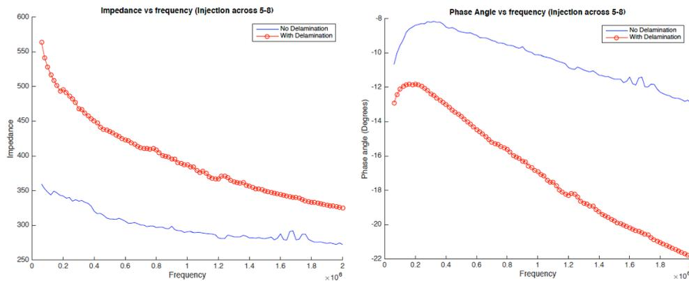
**Figure 2:** Impedance and phase profiles of CFRP samples obtained from the EIS measurements conducted with a current injection along the fiber direction (0°) using electrode pair 5-8 (a) impedance variation, (b) phase angle variation.
