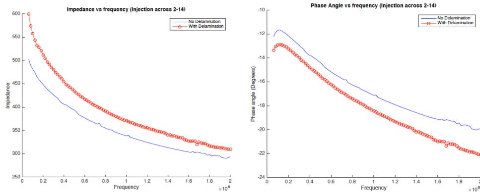
**Figure 3:** Impedance and phase profiles of CFRP samples obtained from the EIS measurements conducted with a current injection perpendicular to the fiber direction using electrode pair 2-14 (a) impedance variation, (b) phase angle variation.
