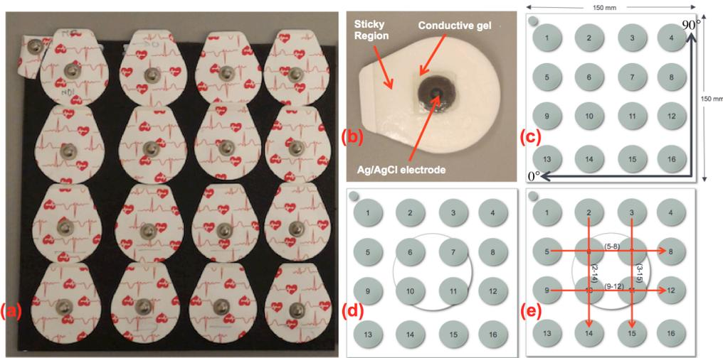
**Figure 1:** ECG electrode arrangements on CFRP samples for their EIS studies (a) 4x4 electrodes array made up of sixteen electrodes (b) a single ECG electrode with Ag/AgCl electrode and conducting gel, (c) geometrical dimension of the samples with electrode positioning, (d) schematic of a sample with a circular delamination, (e) electrode combinations through with the EIS studies are conducted.
