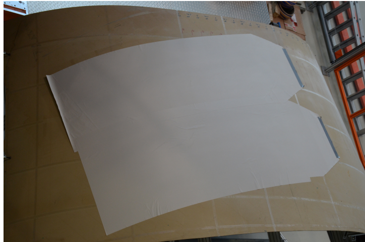
Figure 5. Result of the automated application of two adjacent cuts of LSP material onto convex mould with defined overlap. The overall lay-up quality is good and meets the requirements for the manufacturing of an original panel.
