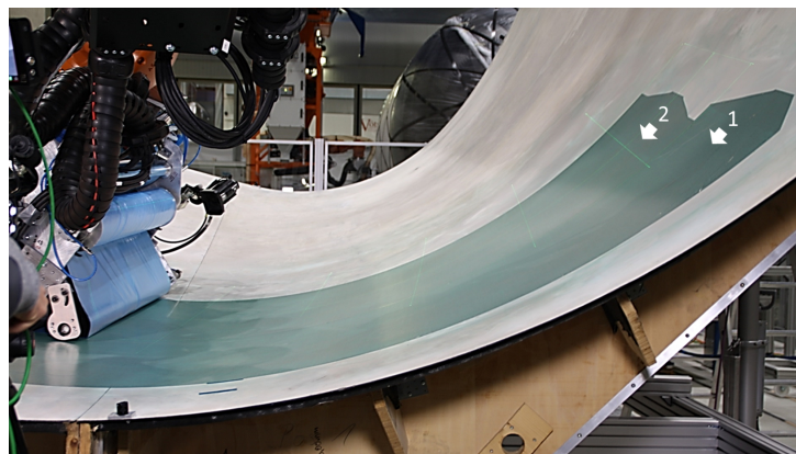
Figure 7. Result of the automated application of two adjacent cuts of LSP material onto concave mould with defined overlap.
