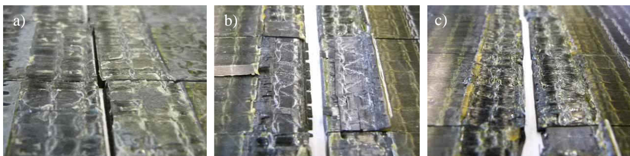
Figure 3. Fracture surfaces of SLS specimens produced with a heating rate of 0.5 K/min a) and 2.6 K/min b) and c).
