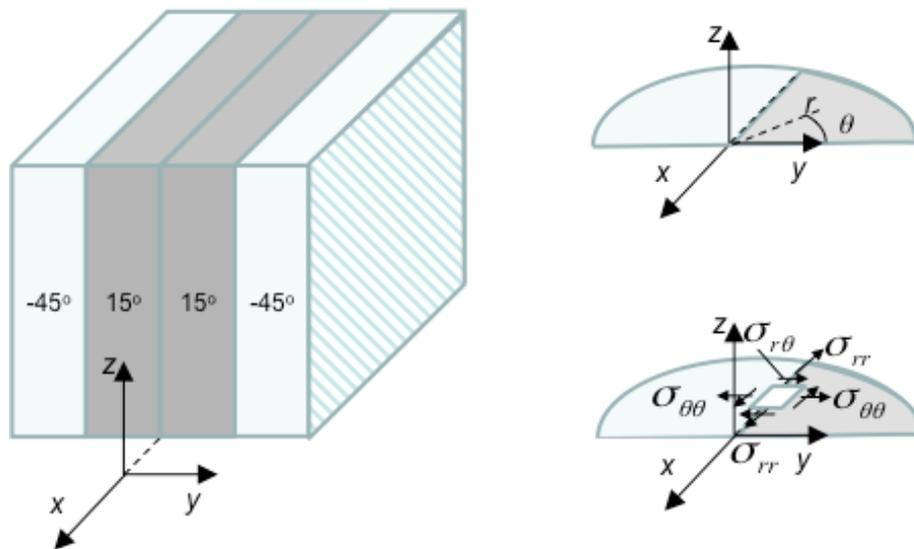
**Figure 1.** Stress state at a boundary point located at the interface of the laminas of a  $[-45, 15]_s$  laminate.
