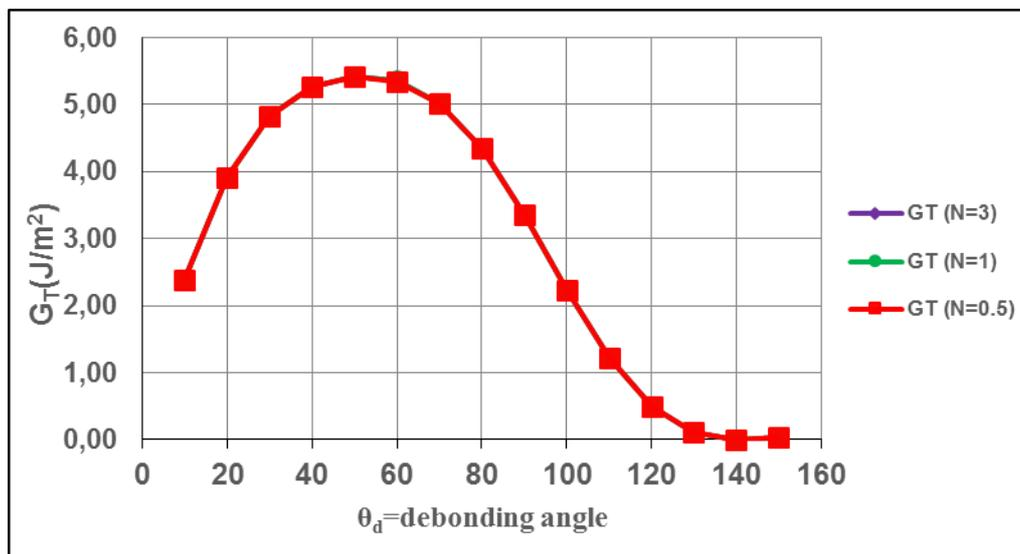
Figure 5. Scale effect on the values of the energy release rate  $G$  corresponding to a debonding crack between fibre and matrix.
