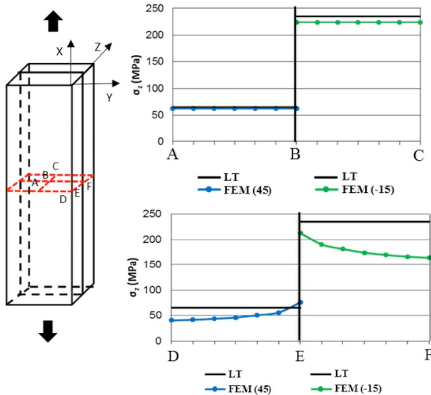
Figure 2. Evolution of longitudinal stress through the thickness of a [-45, 15]<sub>s</sub> laminate.
