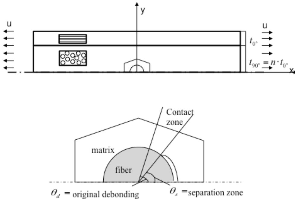
**Figure 3.** Multiscale BEM model of a  $[0_n, 90_n]_s$  laminate with a detail of the micromechanical cell allowing debonding between fibre and matrix.
