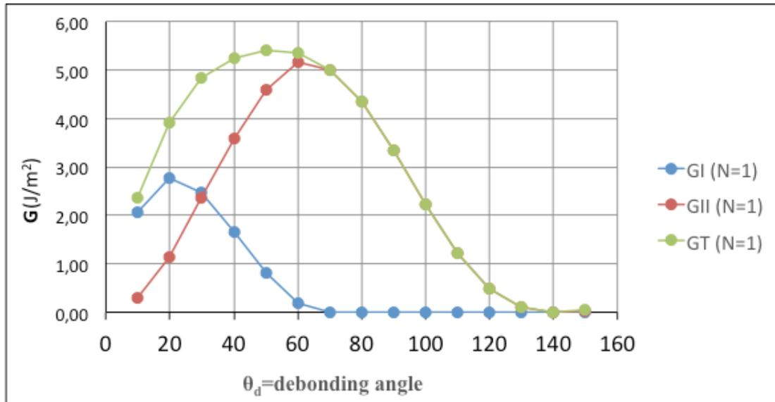
Figure 4. Evolution of  $G$  as a function of the debonding angle.
