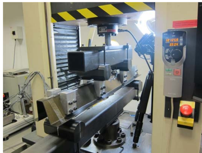
Figure 4. Four-point bend test using Shimadzu Autograph-25 TG universal testing machine
