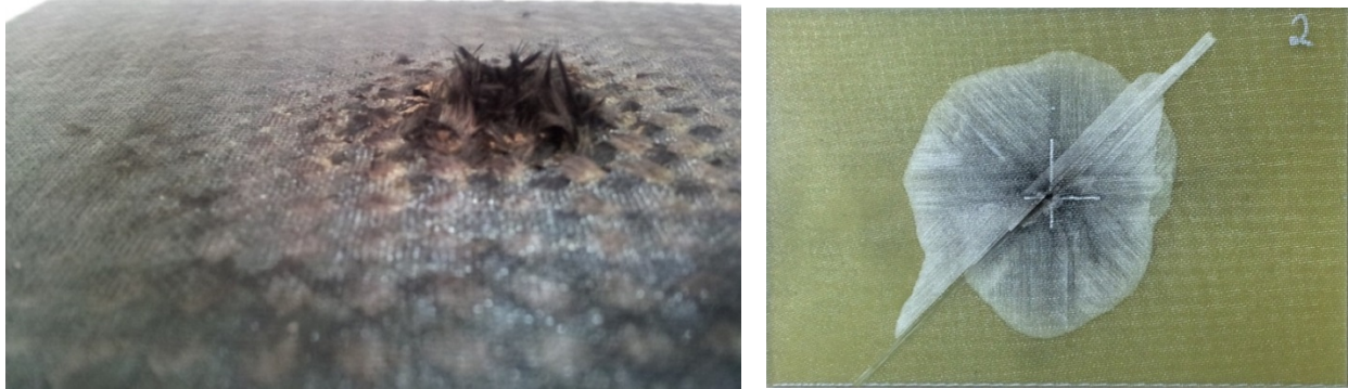
Figure 6 (a) Carbon/epoxy struck by a 90kA current and (b) E-glass/epoxy struck by a 10kA current
