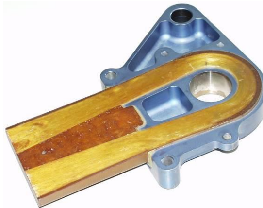
Figure 3. Cut of a rotor blade interface (loop embedded within a titanium fitting)
