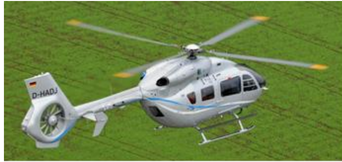
Figure 1. BK117 D-2 (H145) first flight on 18 th March 2011 - figure showing the main rotor blades and Fenestron TM anti torque system
