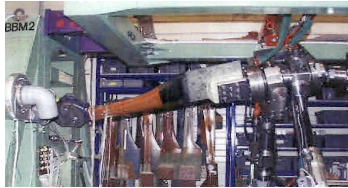
Figure 4. Test set-up for destructive component testing of H145 main rotor blade attachment
