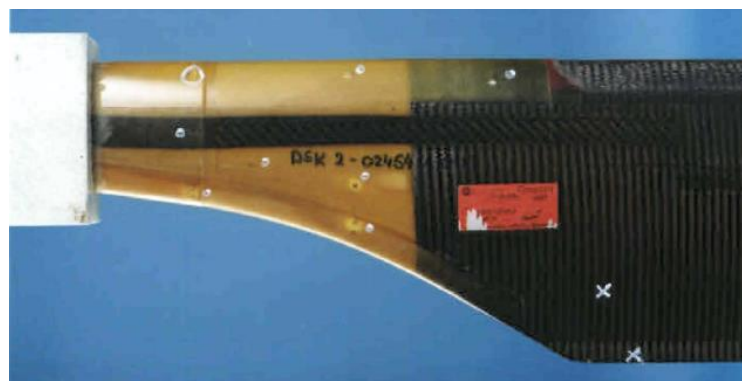
Figure 5: Impact locations on a rotor blade specimen. Different energies are applied on thin (marked by crosses) and thick (marked by dots) zones of the laminate [3]
