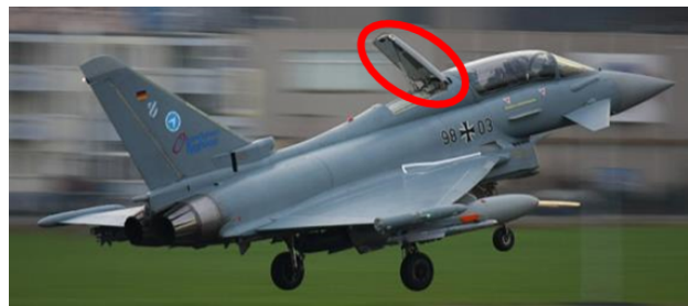
Figure 4. EFA T/S with deflected airbrake (which serves as platform for the R&T activities)
