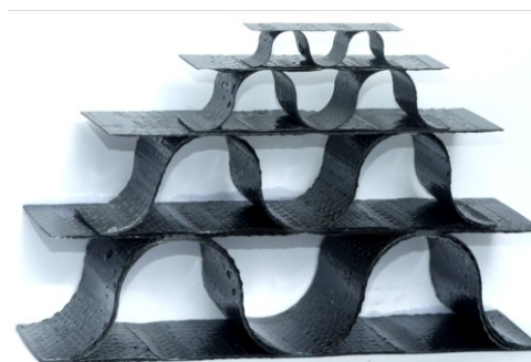
(b) Four scaled sizes of CFRP core ( n=1/4 , n=1/2 , n=3/4 and n=1 ).
