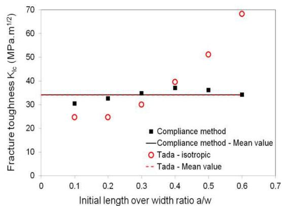
**Figure 8.** Comparison of fracture toughness values as a function of the ratio  $a/w$  of the initial crack length over the specimen width for quasi-isotropic C/PPS laminates obtained from compliance method and semi-empirical formula proposed for SEN isotropic specimens [7].
