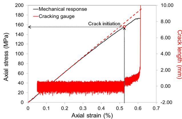
**Figure 6 .** Mechanical response and identification of remote applied stress at crack initiation using a cracking gauge.
