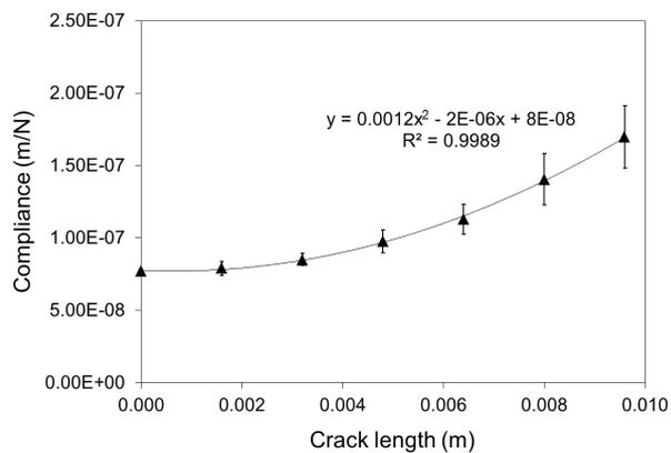
**Figure 7.** Evolution of compliance as a function of the initial crack length for SEN quasi-isotropic C/PPS specimens subjected to tensile loadings at 120°C.
