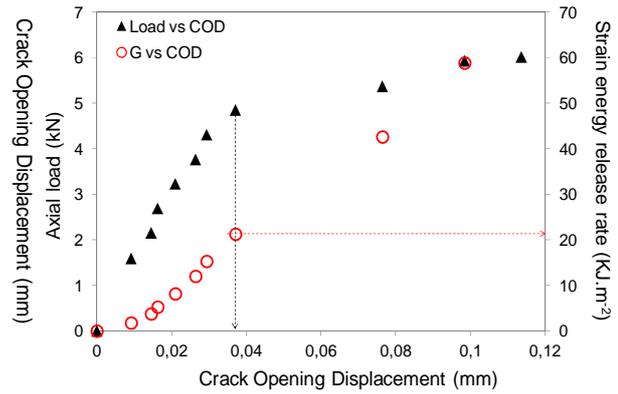
**Figure 5.** Evolution of axial load and strain energy release rate as a function of crack opening displacement in quasi-isotropic laminates at 120°.
