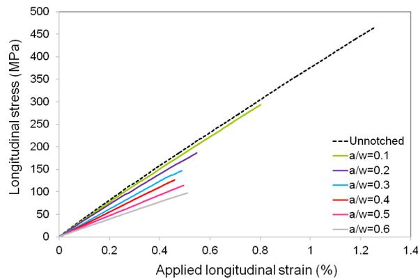
**Figure 1.** Tensile responses of SEN quasi-isotropic C/PPS specimens at 120°C: influence of the ratio  $a/w$  of the initial crack length over the specimen width.
