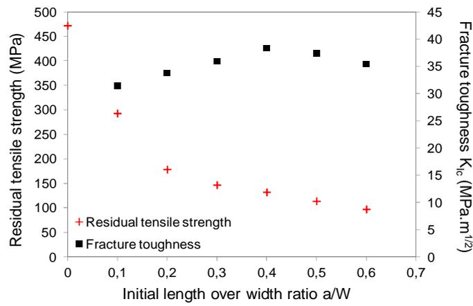
**Figure 9.** Changes in the residual tensile strength of SEN specimens and critical fracture toughness  $K_{IC}$  as a function of the ratio  $a/w$  of the initial crack length over the specimen width obtained from compliance-based method for quasi-isotropic C/PPS laminates at 120°C.
