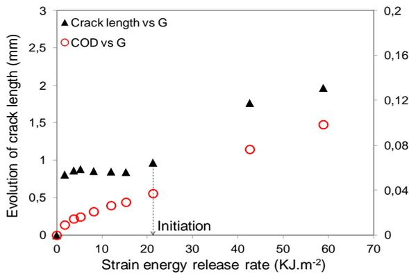
**Figure 4.** Evolution of crack length and crack opening displacement as a function of strain energy release rate in quasi-isotropic laminates at 120°.
