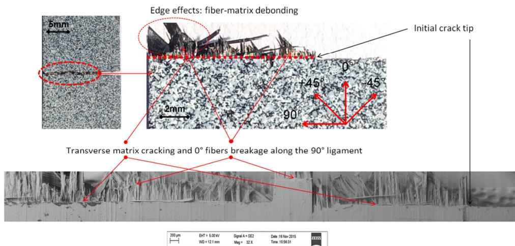
**Figure 2.** Macroscopic and SEM observations of fracture surface for SEN quasi-isotropic C/PPS specimens subjected to tensile loadings at 120°C.
