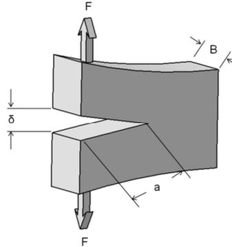
**Figure 3.** Double cantilever beam (DCB) method
