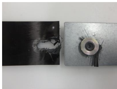
Figure 5. SPR joint after failure
