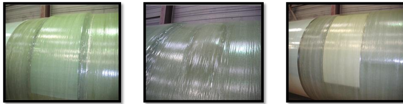
Figure 2. Sandwich materials manufactured using filament winding process by our industrial partner.
