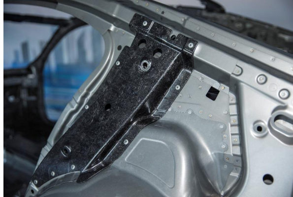
Figure 1. Reinforcement of the C-pillar (right side) made of Carbon Fiber Sheet molding compound (CF-SMC) in the body structure of the BMW 7 (G11/G12) series [1].
