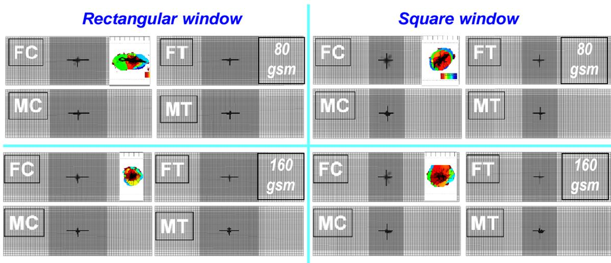
**Figure 5.** Predicted and observed ply damage in laminates impacted at 30 J. (FC/FT=fibre compression/tension, MC/MT=matrix compression/tension)
