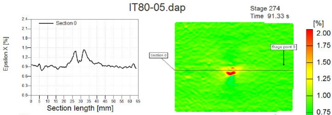
Figure 7. Strain distribution in 80 gsm laminate impacted at 30 J.
