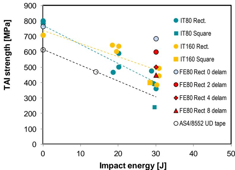
Figure 8. Measured and predicted tensile strength versus impact energy.
