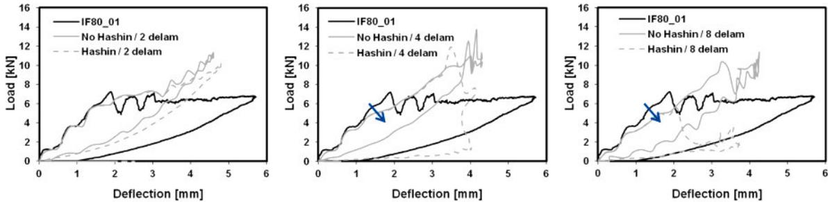
**Figure 4.** Measured and predicted response for 2, 4 and 8 delaminations without/with inplane damage.
