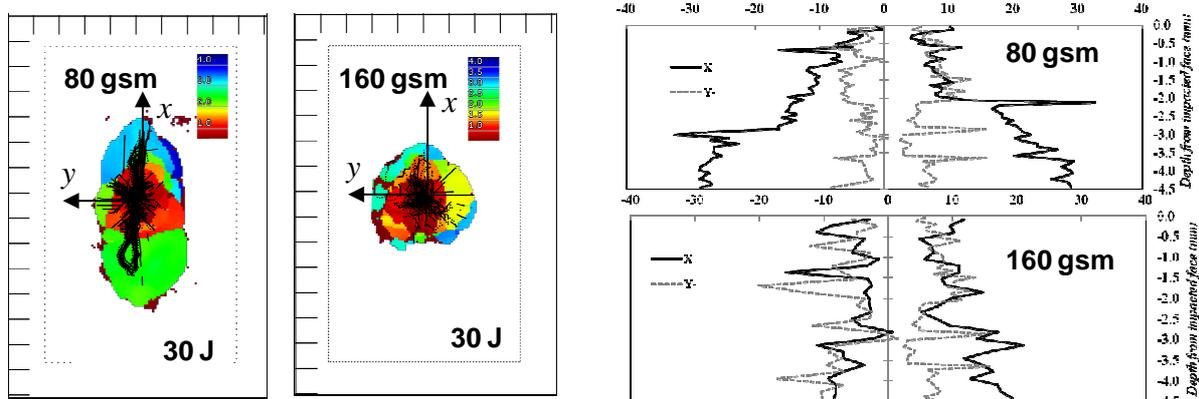
**Figure 3.** In-plane and through-thickness distribution of fibre cracks in the laminates.
