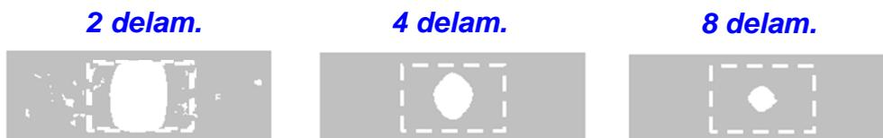
**Figure 6.** Predicted delaminations in an 80 gsm laminate impacted at 30 J.
