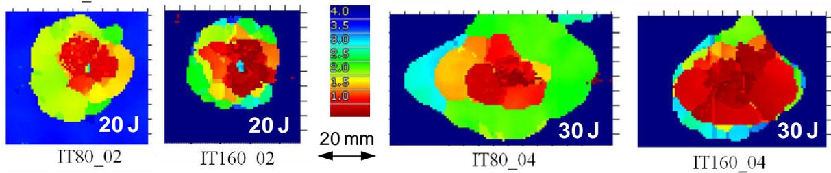
**Figure 2.** Differences in delaminations in 80 and 160 gsm laminates impacted at 20 and 30 J.
