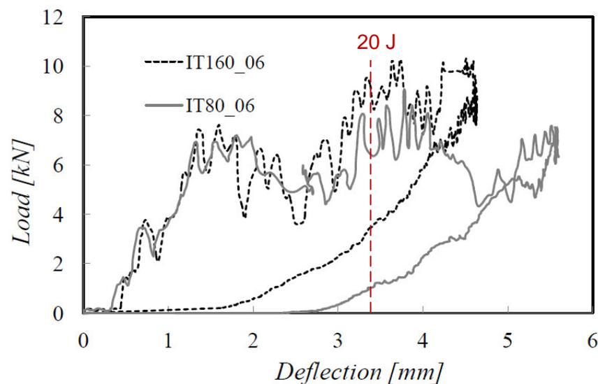
**Figure 1.** Typical load-deflection for an 80 and 160 gsm laminate impacted at 30 J.
