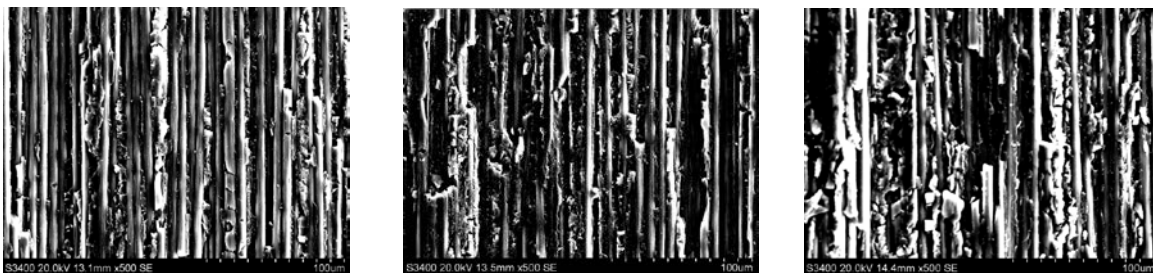
(a) A=7\mu\text{m} f=20.6\text{KHz} A \times f=144200 (b) A=5\mu\text{m} f=20.5\text{KHz} A \times f=102500 (c) A=0 f=0 A \times f=0
