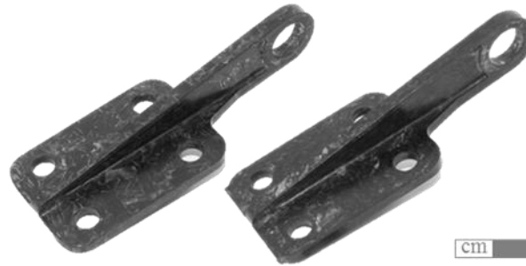
Figure 2. Compression molded door hinge demonstrator used for this study, the part on the left is made from chopped tapes, the part on the right is made from recycled fragments
