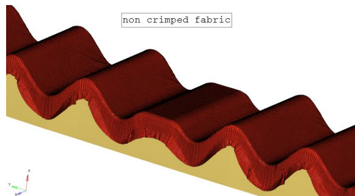
Figure 5. Draping of \pm 45^\circ NCF ply
