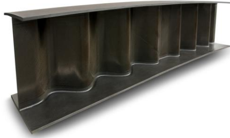
Figure 1. Sine Wave Spar, 2.5m long 1:1 scale segment of a heavily loaded wing spar made from CFRP, Ref. [2]
