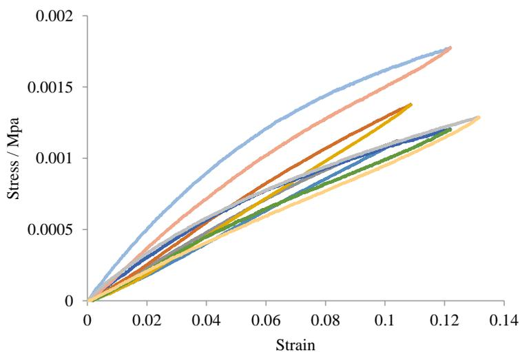
**Figure 3:** An example of the fifth cycle recorded in the cyclic compression tests performed on 5 different samples of each foam system. The energy dissipation was calculated as the area between the compression and returning curve and the standard deviation was taken over the 5 samples.
