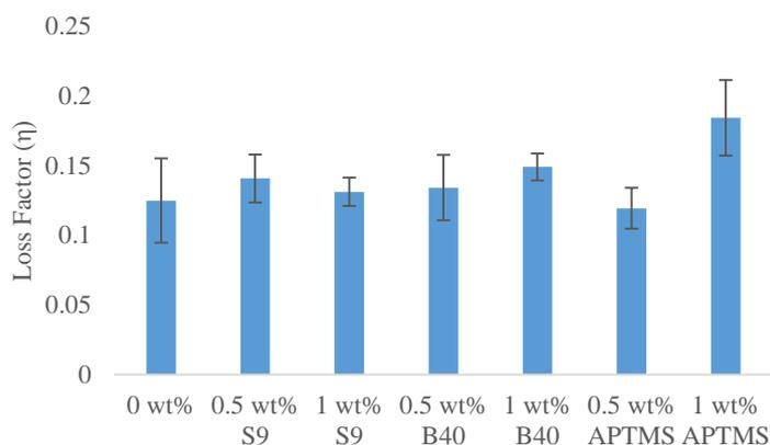
**Figure 5:** Loss Factor ( $\eta$ ) for each composite system. Measured as the ratio of the energy dissipation over the work applied to the system. The error was calculated as the standard deviation over 5 samples.
