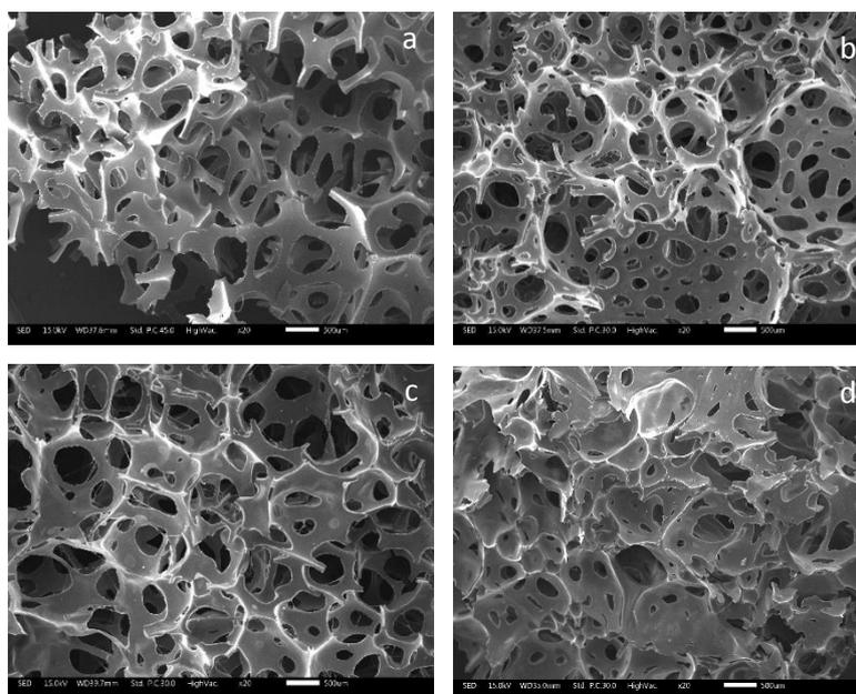
**Figure 1:** SEM micrographs of polyurethane foam with: a) 0 wt% clay, b) 1 wt% S9 sepiolite, c) 1 wt% B40 sepiolite and d) 1 wt% silane modified S9. Each sample has been magnified 20 times in the above micrographs.
