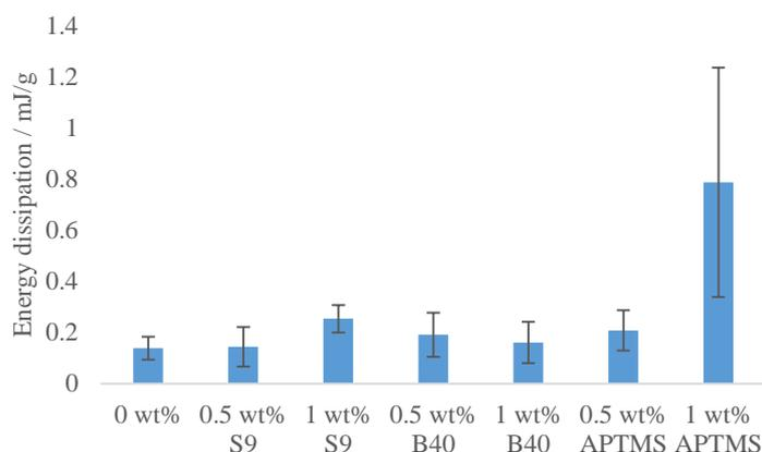
**Figure 4:** Energy Dissipation per gram values for each composite system. This is calculated as the area under the curve of the fifth cycle of each sample, divided by the sample density. The error was calculated as the standard deviation over 5 samples.
