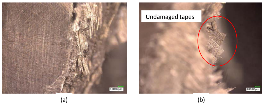
Figure 3. Microscope observation on fracture part of UT-CTT: (a) dry and (b) wet.
