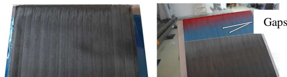
Figure 6. Photo of the frontside (left) and backside (right) of the corner during lay-up of 90° specimens with highlighted too hot and too cold regions
