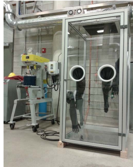
Fig. 1: (a) Union Process attritor mill used at CANMET Materials Lab, (b) enclosure to safely handle the alloyed powder
