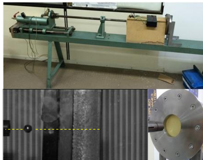
Figure 3. Air-gun apparatus, tubular fixture and sphere trajectory.
